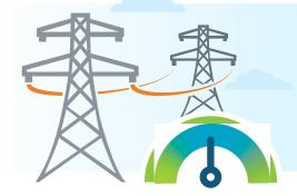
Reactive power helps support appropriate voltages on the transmission system to allow for the movement of real power across transmission lines.
