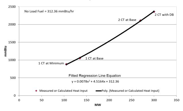
Each diamond in the graph above is a design heat input data point obtained from the original equipment manufacturer or calculated by heat balance. A regression analysis was performed on the design data to obtain the unit's Heat Input curve as a function of unit output levels with natural gas as a fuel:
