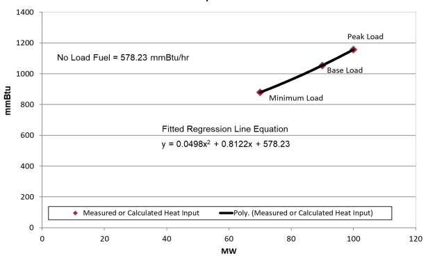
Each diamond in the graph above is a design heat input data point obtained from the original equipment manufacturer or calculated by heat balance. A regression analysis can be performed on the design data to obtain the unit's Heat Input curve as a function of various unit output levels with natural gas as a fuel:
