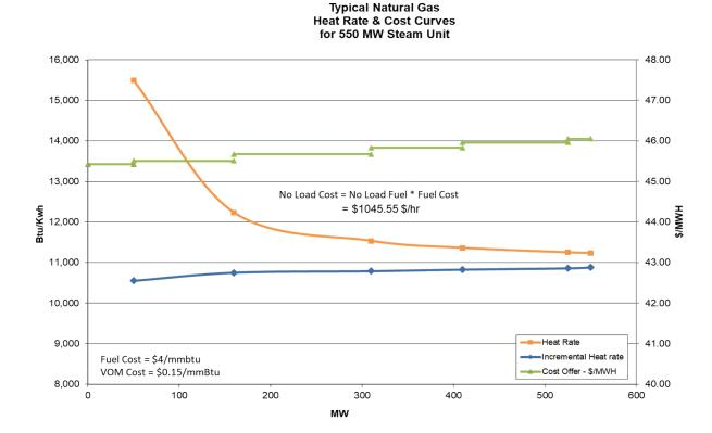
To avoid making adjustments to the no-load cost, first calculate the unit's Incremental Cost (\$/MWh) at various outputs using the derivative of the Heat Input Curve:
