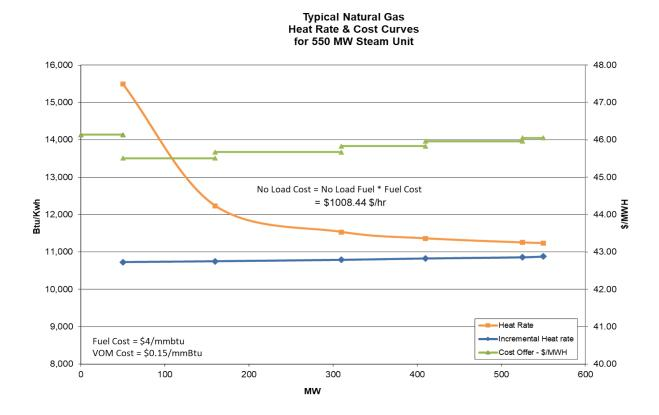
The o-load cost was then raised to \$1007.76 until the first increment of the cost offer was less than \$1/MWh below the second increment, producing a monotonically increasing curve in the graph below:
