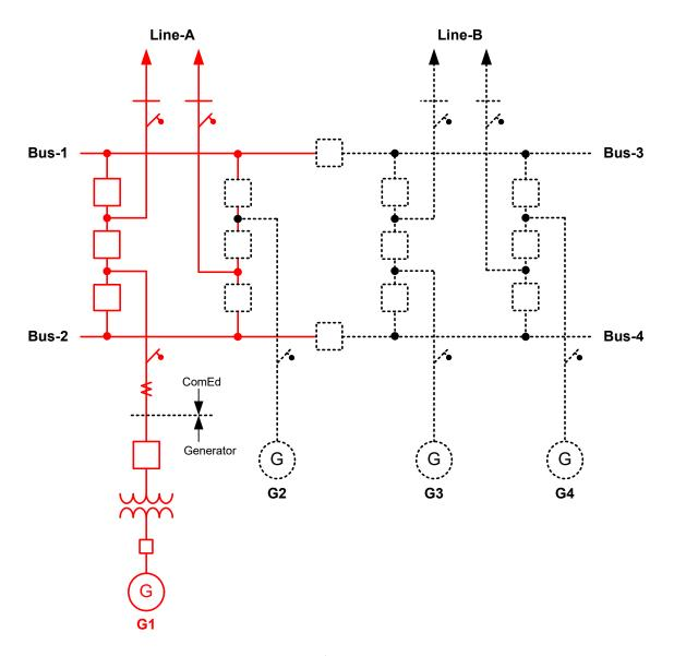
Figure-a: Interconnection of 1<sup>st</sup> Generator at a Generation Hub (G1 on Line-A)
