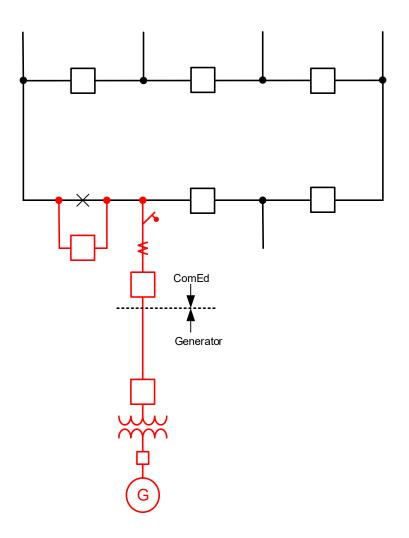
Figure-3.1.1: Generator interconnection to an existing nuclear station
