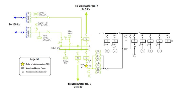
The Point of Interconnection is at the jaws (the Interconnection Customer side) of the 34.5 kV disconnect switch mounted on the AEP owned metering structure located within the fenced area comprising AEP's Reusens station. The Interconnection Customer owns the conductors up to the mechanical connection at the meter structure customer-side receiving standoff post-insulators as well as the tap conductor to the disconnect switch jaws.
