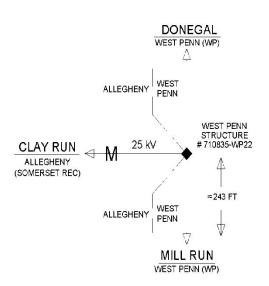
= CLAY RUN DELIVERY POINT LOCATED WHERE ALLEGHENY'S LINES TERMINATE ON WEST PENN'S STRUCTURE #710835-WP22
