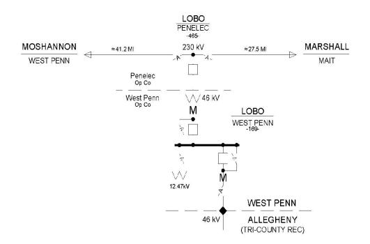
= DELIVERY POINT IS WHERE ALLEGHENY'S LINE TERMINATES ON STEEL STRUCTURE INSIDE WEST PENN SUBSTATION
