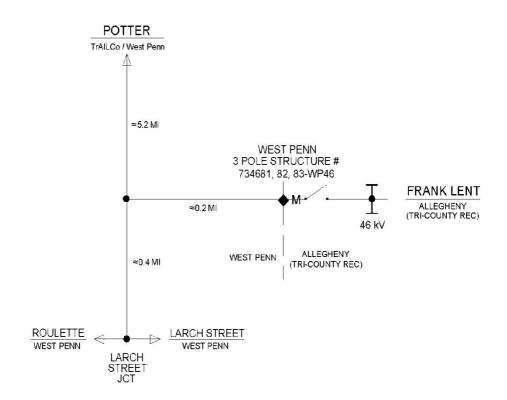
◆ = FRANK LENT DELIVERY POINT LOCATED WHERE ALLEGHENY'S LINES TERMINATE ON WEST PENN'S 3 POLE STRUCTURE 734681, 82, 83-WP46, OUTSIDE THE SUBSTATION
