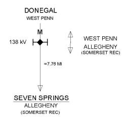
= SEVEN SPRINGS DELIVERY POINT LOCATED WHERE ALLEGHENY'S LINES TERMINATE ON WEST PENN'S SUBSTATION DEAD-END STRUCTURE
