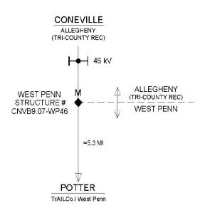
= CONEVILLE DELIVERY POINT LOCATED WHERE ALLEGHENY'S LINES TERMINATE ON WEST PENN'S STRUCTURE CNVB9.07-WP46, OUTSIDE THE SUBSTATION
