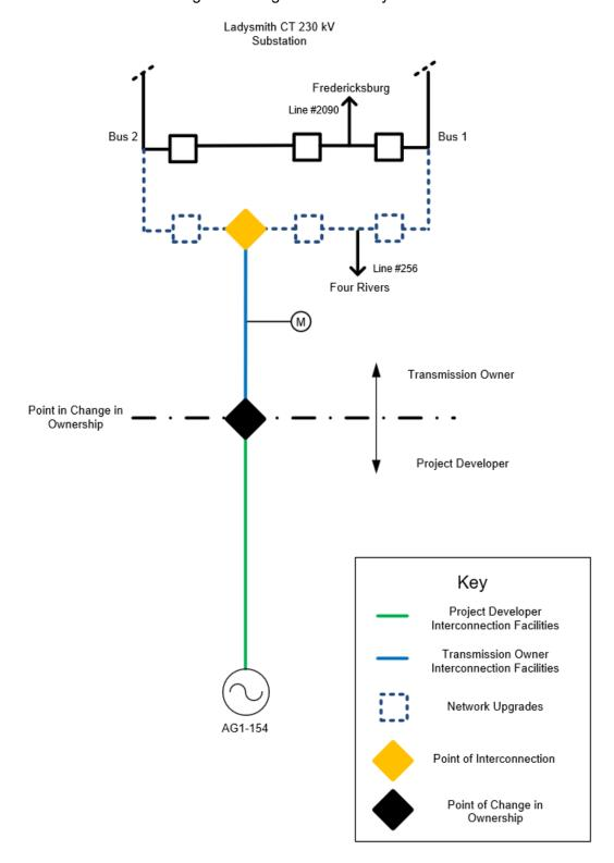
Attachment #2: Substation General Arrangement
