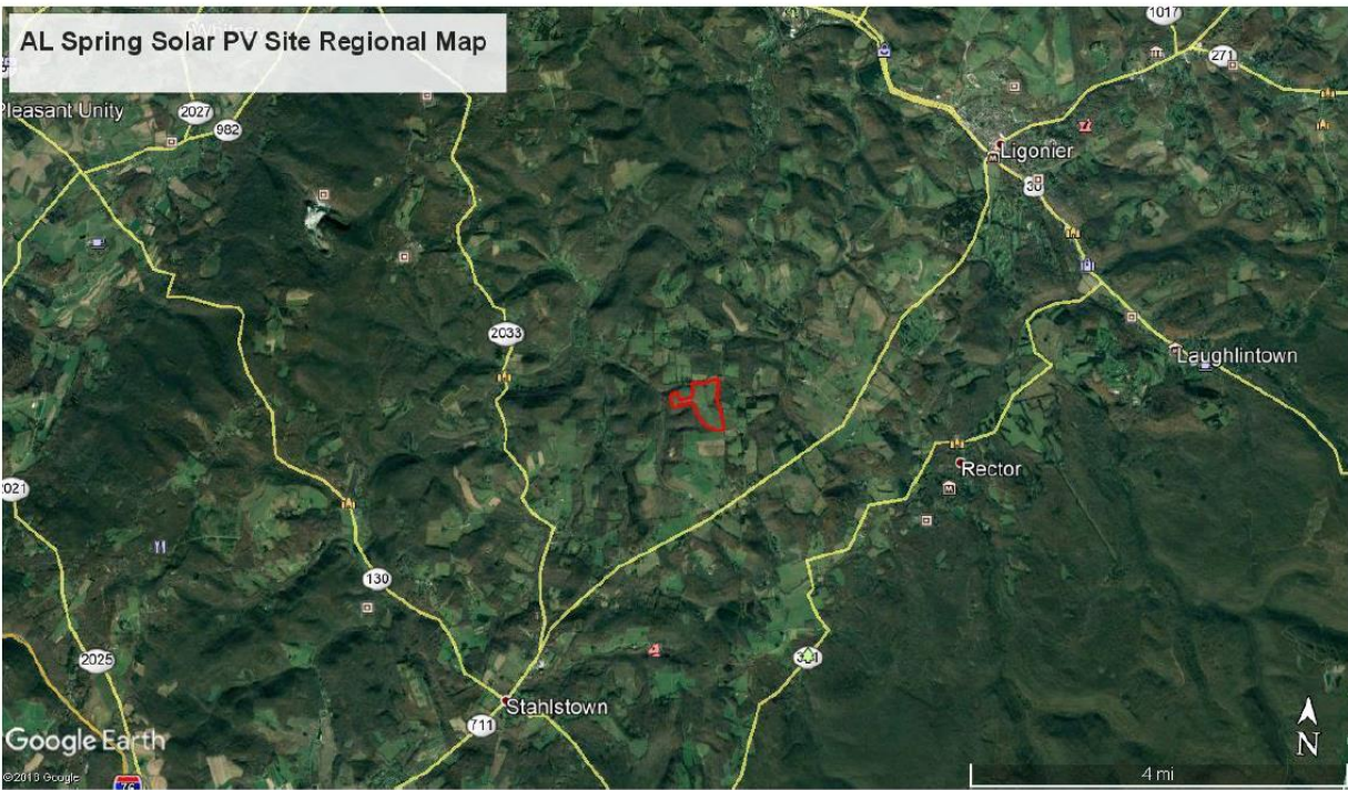
AL Spring Regional Map with Solar PV site in RED. POI on 25kV segment running from Ligonier to Stahlstown, PA.
