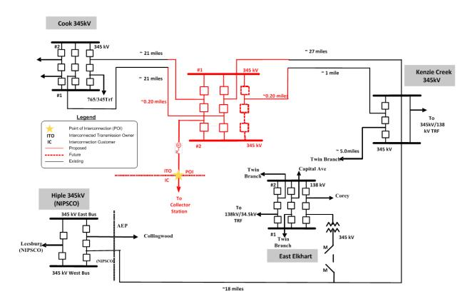
The Point of Interconnection is at the first structure outside of the new 345 kV switching station with the Interconnected Transmission Owner owning the first span of conductors out of its switching station and the Interconnection Customer owning the first structure and remaining structures and conductors back to its generation collector station.
