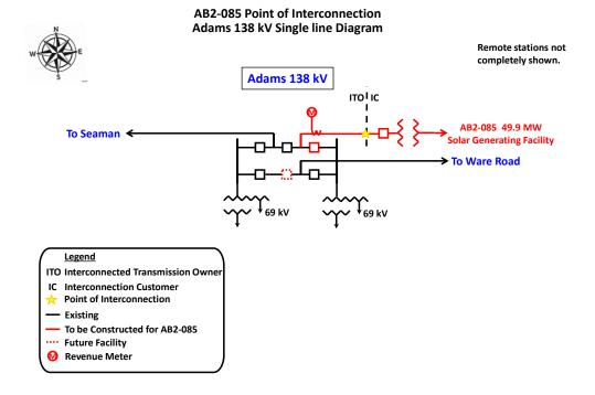
The Point of Interconnection is at the first (dead-end) structure outside of the Adams 138 kV Station fence. AEP owns the span from the Adams 138 kV Station to the dead-end, including the jumpers and structure at the dead-end. Interconnection Customer owns the span and structures from the dead-end to the AB2-085 generation collector station.
