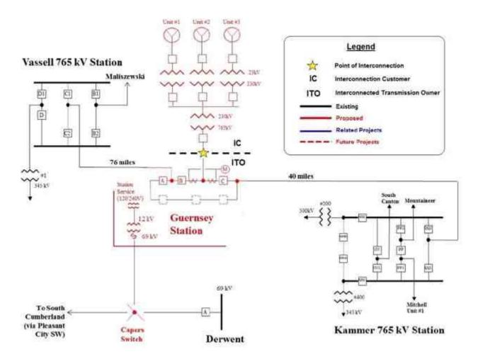
The Point of Interconnection is at the first structure outside of the new 765 kV switching station with AEP owning the first span out of its switching station and the Interconnection Customer owning the first structure and remaining conductors back to its generation collector station.
