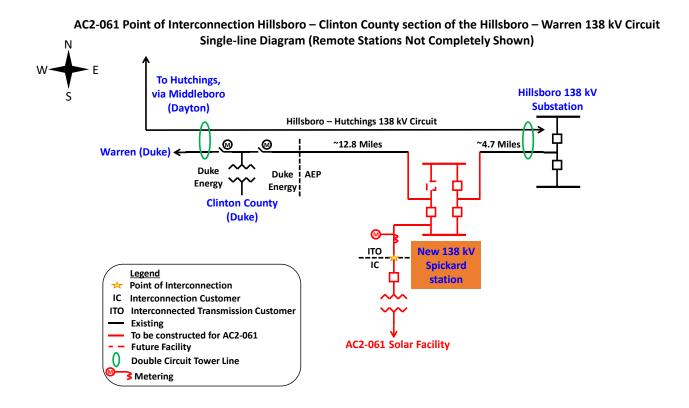
The Point of Interconnection is the first structure outside of AEP's proposed Spickard 138 kV Station (such structure being the station dead end structure located inside the Interconnection Customer's Collector Substation). The Interconnected Transmission Owner will own the span of conductors from the proposed Spickard 138 kV Station to the Interconnection Customer Collector Station dead end structure, with the Interconnection Customer owning said dead end structure.
