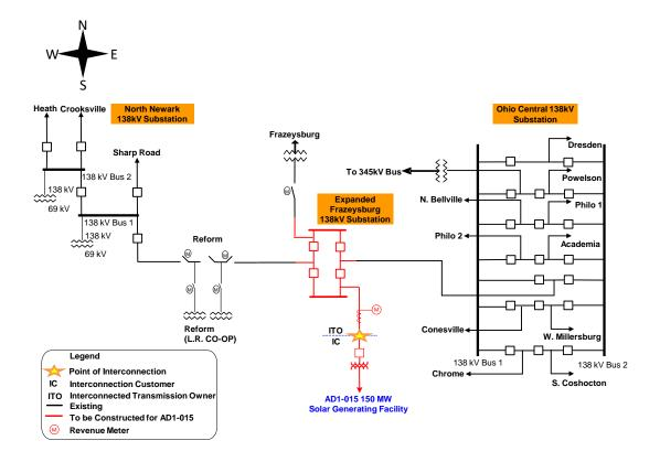
The Point of Interconnection is the structure located in Interconnection Customer's 34.5-138 kV collector substation with the Interconnected Transmission Owner owning the span of conductors out of its station, and the Interconnection Customer owning the structure.
