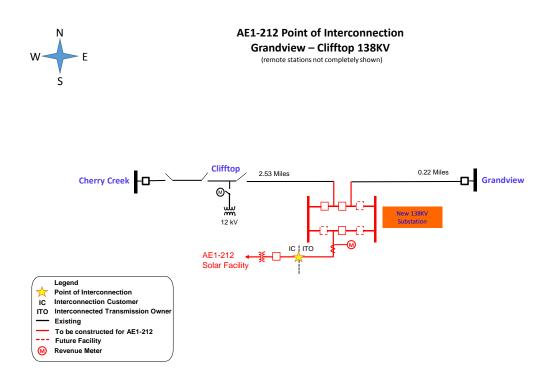
The Point of Interconnection ('POI') is at the first structure outside of the Interconnected Transmission Owner's proposed 138 kV station (such structure being located in the Interconnection Customer's Collector station) with the Interconnected Transmission Owner owning the first span of conductors, and the Interconnection Customer owning the first structure.
