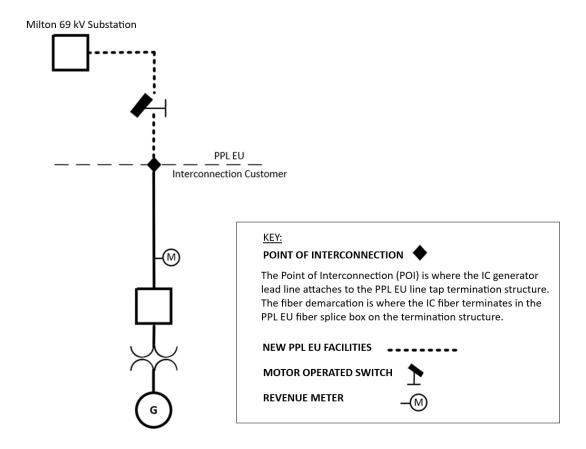
For purposes of this Single-Line Diagram, Interconnection Customer is abbreviated IC.
