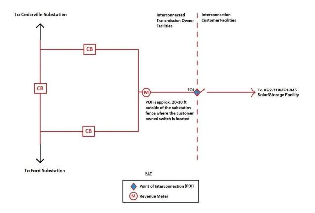
AE2-318/AF1-045 (new facilites to be constructed shown in red)
