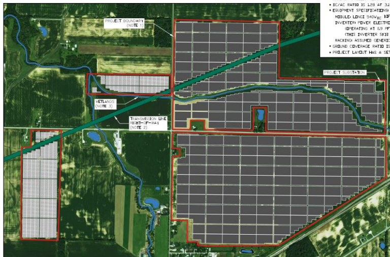
205 MWAC MAXIMUM FACILITY OUTPUT SITE LAYOUT
