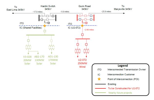
The Point of Interconnection ("POI") will be on the first structure outside of ITO's new 345 kV switching station with the ITO owning the first span of conductors required to interconnect the IC's Facility, and IC owning all structures and remaining conductors to the IC's generation station.
