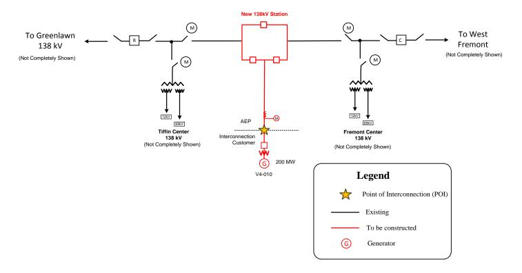
The Point of Interconnection will be at the first structure outside of the new 138 kV transmission switching station with AEP owning the conductors to the first structure, and Interconnection Customer owning the structure and all remaining facilities back to the generation collector station.
