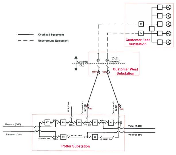
Note: The Point of Interconnection(s) will be the customer side of the line disconnect switches in the Customer West substation
