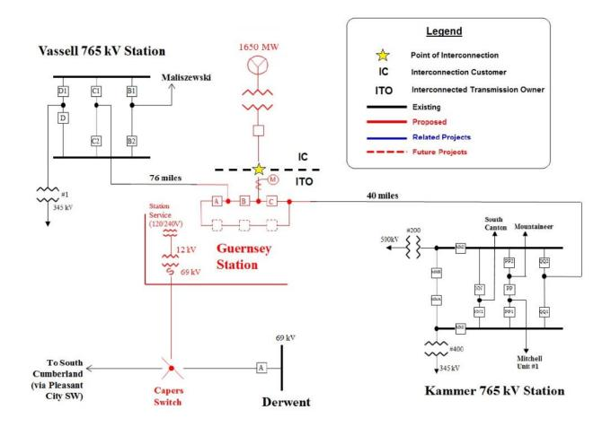
Figure 2: Point of Interconnection (Guernsey 765 kV, served via AEP Kammer-Vassell 765kV circuit)
