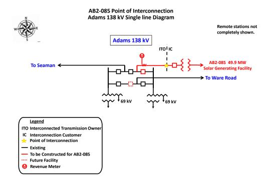
The Point of Interconnection ("POI") is at the first (dead-end) structure outside the Adams 138 kV station fence. AEP owns the span from the Adams 138kV station to the Dead-end, including the jumpers and structure at the Dead-end. Community Energy owns the span connecting to the POI, and the 138kV generator lead line and remaining structures back to the AB2-085 generation collector station.
