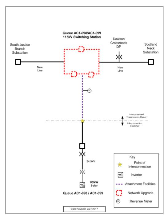
Attachment 2. AC1-098\_099 Switching Station General Arrangement
