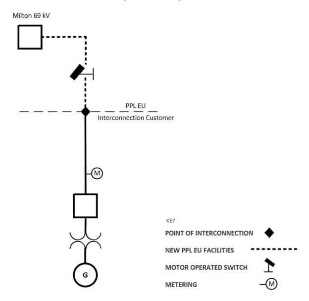
The Point of Interconnection (POI) is where the IC generator lead line attaches to the PPL EU line tap termination structure. The fiber demarcation is where the IC fiber terminates in the PPL EU fiber splice box on the termination structure.
