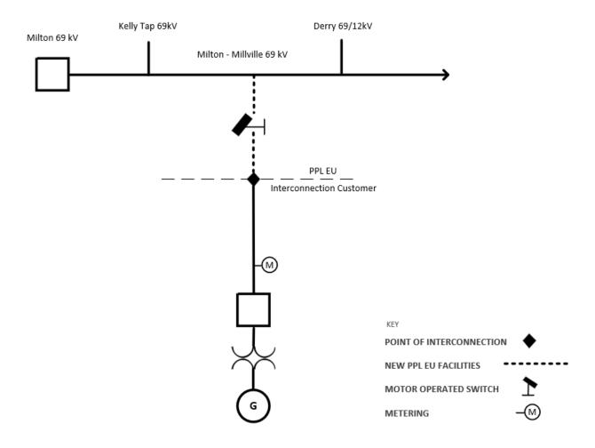
The Point of Interconnection (POI) is where the IC generator lead line attaches to the PPL EU line tap termination structure. The fiber demarcation is where the IC fiber terminates in the PPL EU fiber splice box on the termination structure.
