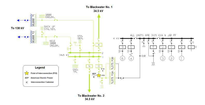
Figure 3: PJM Queue AB2-109 Reusens Station and Hydro Dam
