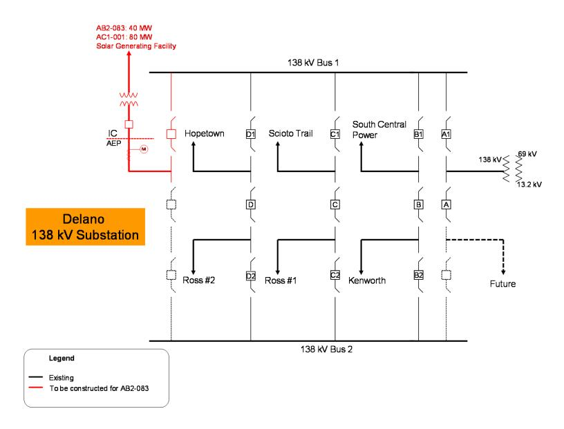
Figure 2: Point of Interconnection (Delano 138 kV Substation)
