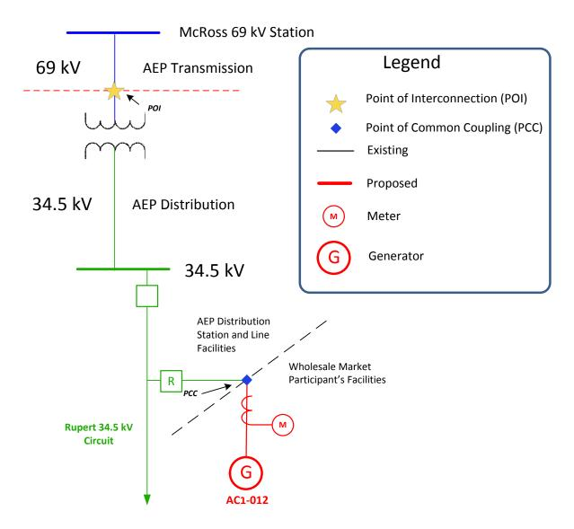
The Point of Interconnection with the transmission system is at Transmission Owner's McRoss 69 kV Station at the Transmission Owner's 69 kV disconnect switch. The point of common coupling (PCC) with the local distribution system will remain at AEP's distribution primary meter facility on the Wholesale Market Participant's premise.
