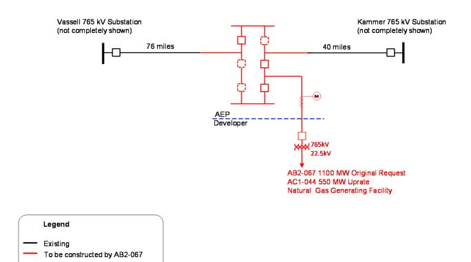
Figure 2: Primary Point of Interconnection (Kammer – Vassell 765 kV Line)
