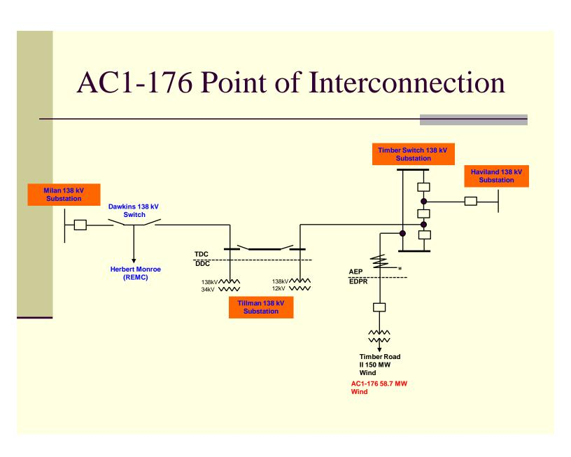
Figure 2: Point of Interconnection (Timber Switch 138 kV Substation)
