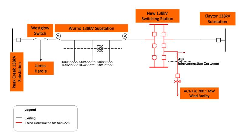
Figure 2: Point of Interconnection (Wurno – Claytor 138 kV)
