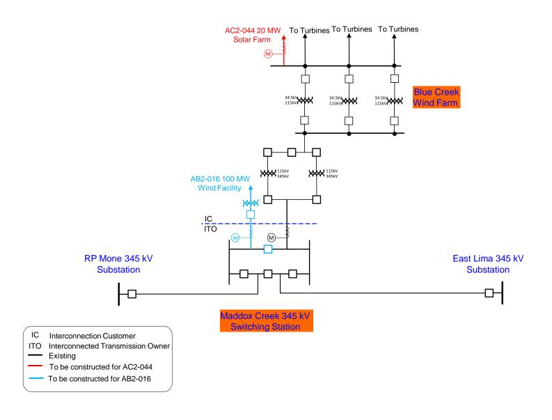
Figure 2: Point of Interconnection (Blue Creek 34.5 kV Collector Station)
