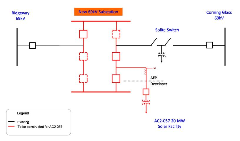
Figure 2: Primary Point of Interconnection (Ridgeway - Solite 69 kV)
