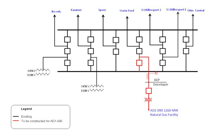
Figure 3: Secondary Point of Interconnection (Muskingum River – W. Millersport #2 345 kV)
