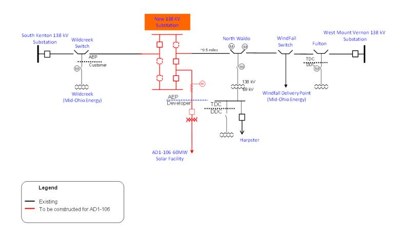
Expanded North מסמן Waldo 138 KV Substation West Mount Vernon 138 kV WindFall Substation Fulton Switch South Kenton 138 kV Wildcreek Substation New 138kV Switching Switch station Windfall Delivery Point AEP (Mid-Ohio Energy) Developer Wildcreek (Mid-Ohio Energy) Legend Existing AD1-106 60MW To be constructed for AD1-106 Solar Facility
