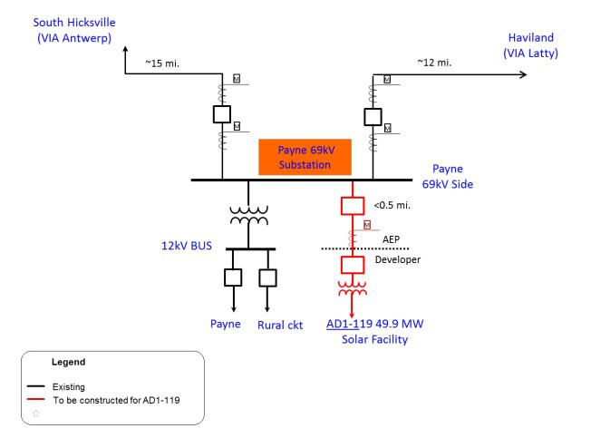
Figure 3: Secondary Point of Interconnection (New 69 kV Substation)
