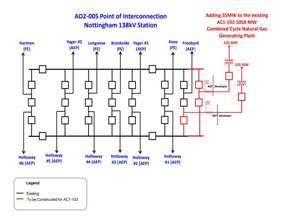
Figure 2: Point of Interconnection (Nottingham 138 kV Substation)
