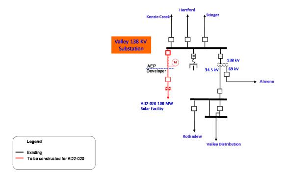
Figure 2: Primary Point of Interconnection (Valley 138 kV)
