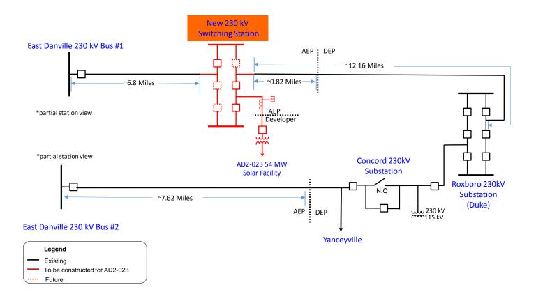
Figure 4: Secondary Point of Interconnection (East Danville - Roxborough 230 kV)
