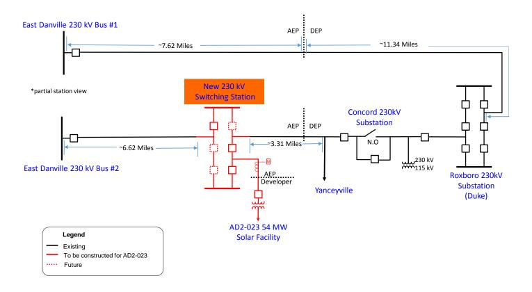
Figure 2: Primary Point of Interconnection (East Danville – Yanceyville Tap 230 kV)
