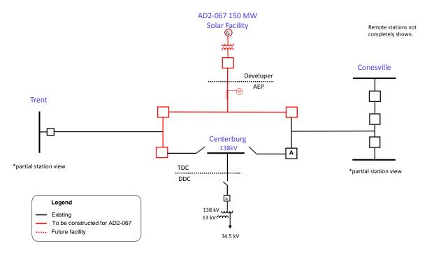
Figure 2: Primary Point of Interconnection (Centerburg 138 kV Substation)
