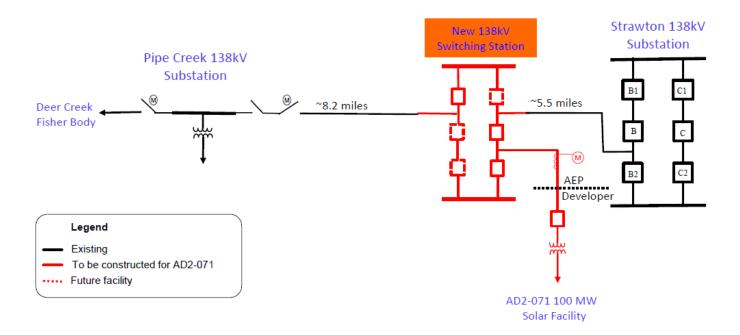
Figure 2: Point of Interconnection (Pipe Creek – Strawton 138 kV)
