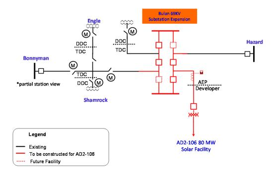
Figure 3: Secondary Point of Interconnection (Shamrock - Bulan 69kV)
