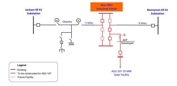
Figure 3: Secondary Point of Interconnection (Chavies 69 kV)
