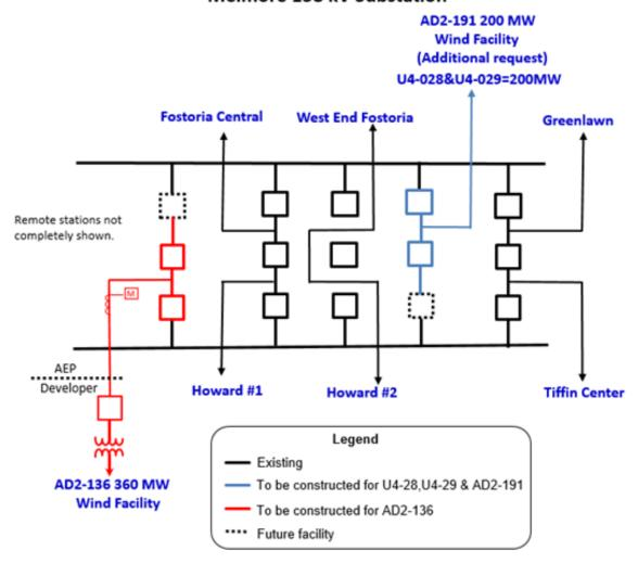
Figure 3: Secondary Point of Interconnection (Melmore 138 kV)
