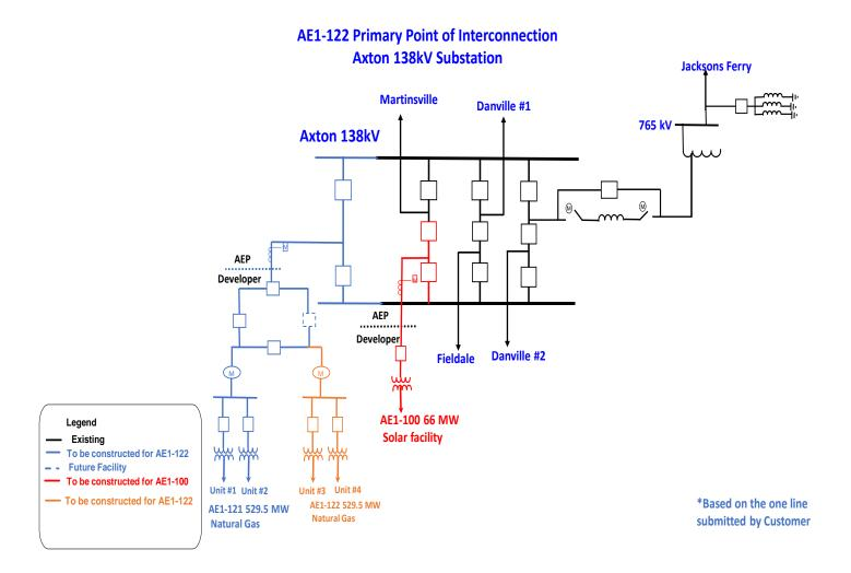
Figure 2: Primary Point of Interconnection (Axton 138kV)
