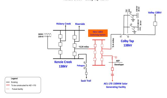
Figure 3: Secondary Point of Interconnection Kenzie Creek 138 kV Substation Single-Line Diagram
