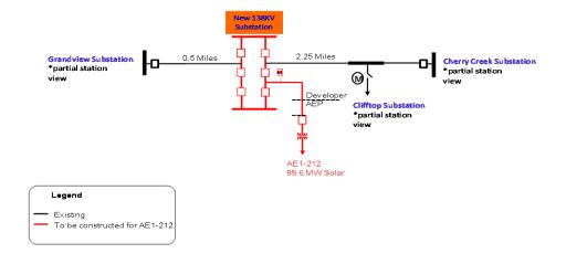
Figure 3: AE1-212 Secondary Point of Interconnection (Grandview – Bradley 138 kV)
