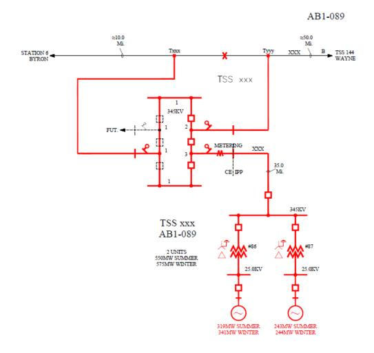
Figure 1. Single Line Diagram
