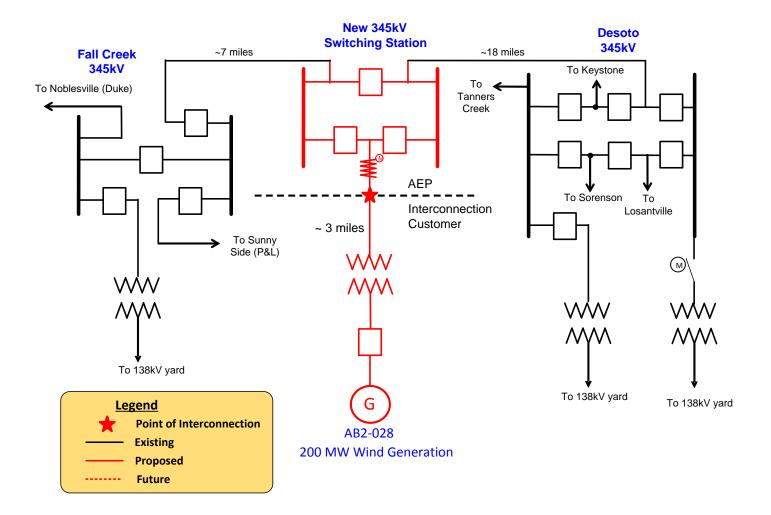
Figure 2: Point of Interconnection (Desoto – Fall Creek 345 kV)
