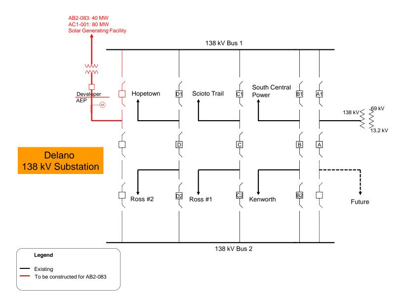
Figure 2: Point of Interconnection (Delano 138 kV Substation)
