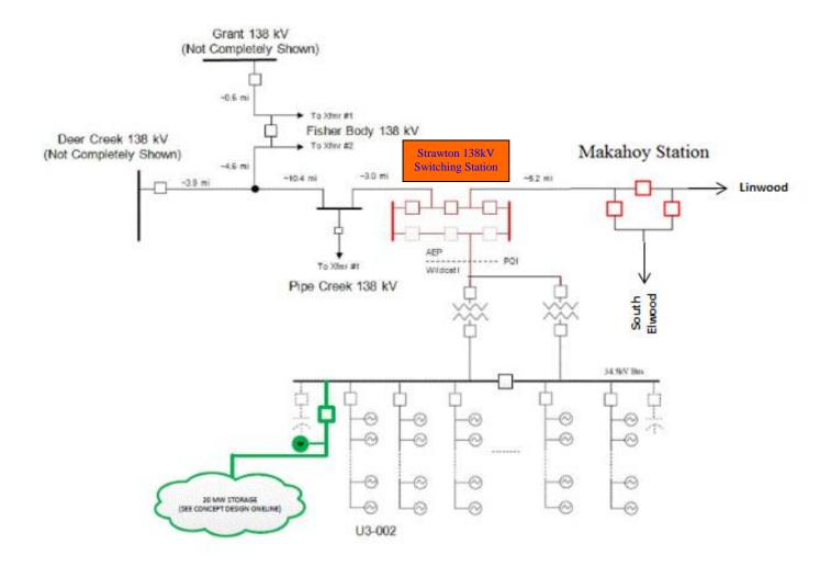
Figure 2: Point of Interconnection (Strawton 138 kV Switching Station)
